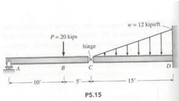
Problem 4: Draw the shear and moment diagrams, label the maximum values of shear and moment, and locate points of inflection.
