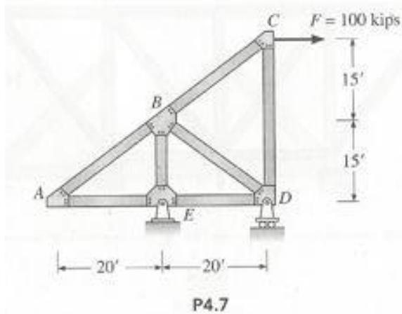
Problem 2: Determine the forces in all truss bars using method of sections. Indicate tension or compression.
